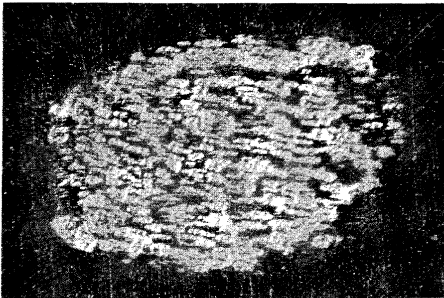
b. after welding time t = 10 ms.
