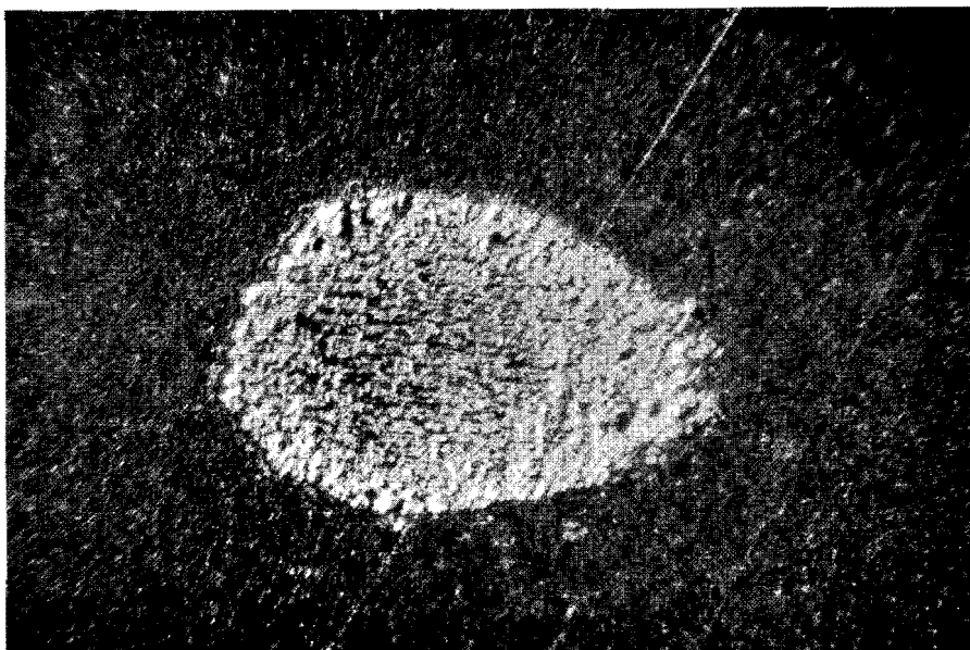
b. after welding time t = 40 ms.
