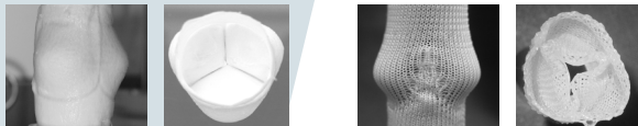
Figure 2. a) an electrospun scaffold, seen from the side, b) seen from the bottom, c) a knitted scaffold pulled over a mould and d) released from the mould, covered with fibrin.
