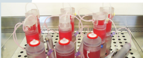
Figure 4. The bioreactor; in the back six culture chambers with valves and in the front three medium vessels.
