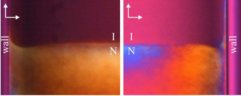
Figure 6.5: Polarisation micrographs of an isotropic-nematic (I-N) interface of charge-stabilised gibbsite platelets, dispersed in a 10^{-2} M NaCl solution. Indicated are the orientations of the polarisers (arrows at right angles in the top left-hand corner) [202].
