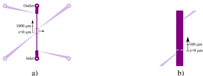
Figure 6.1: Schematic top view representation of the channel layout, a) entire channel, b) magnification of the constriction. The main channel with the constriction is in the center (dark colour). The diagonal channels (light colour) are connected to pressure sensors or dead ends.
