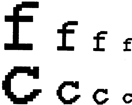
Figure 4: Examples of some discrete letters implemented in the computer to simulate the Courier 10 type font, shown for four sizes. The letters were framed in matrices of 16 \times 32 pixels. If the height of the letters decreases, the frayed effect of discretising can be seen to diminish.
