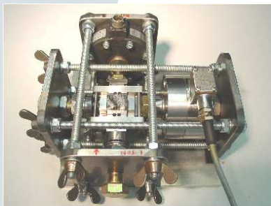
Figure 2 Prototype of discrete die, surface dimensions: 20x30 mm, forming pressures up to 5 ton.
