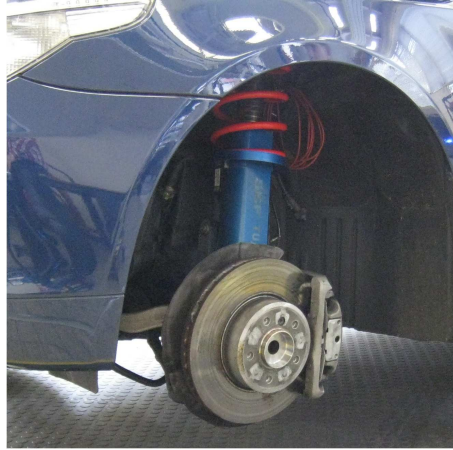
Figure 7.29: Installation of the active suspension system within the BMW 530i.
