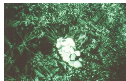
Fig. 5 An optical microscopy picture of microtomed slice taken from the cross-section of a pull-out sample showing the presence of (partial) trans-crystallinity around Duralin flax fibre cells bundle.
