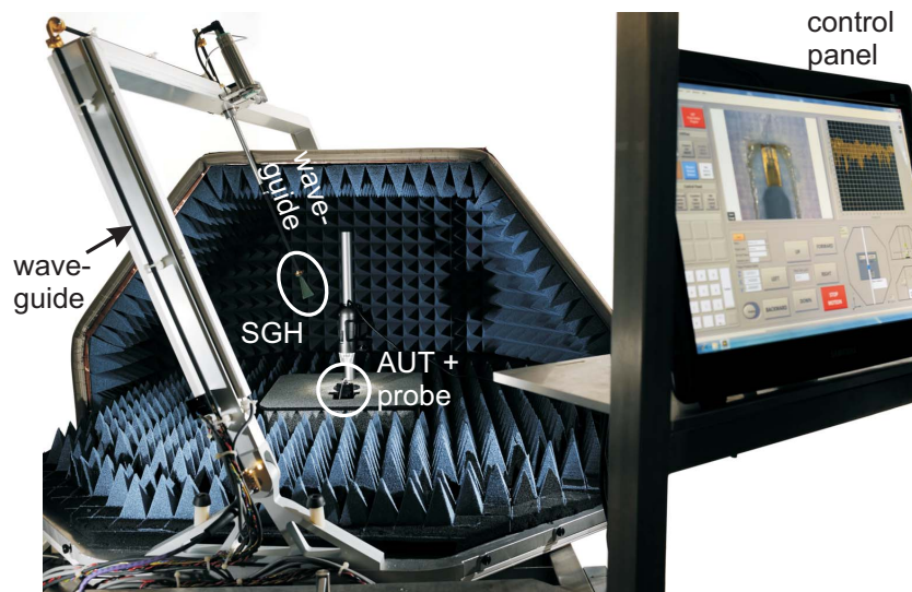
(a) Photograph of the mm-wave anechoic chamber (chamber opened to show inside).
