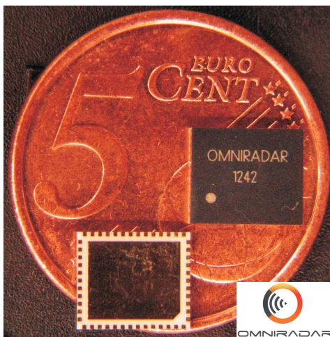
(b) Packaged chips from the top side (top right) and bottom side (bottom left).
