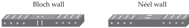
Figure 5.15: Schematic representation of Bloch domain wall (left) and Néel domain wall (right) in thin films.
