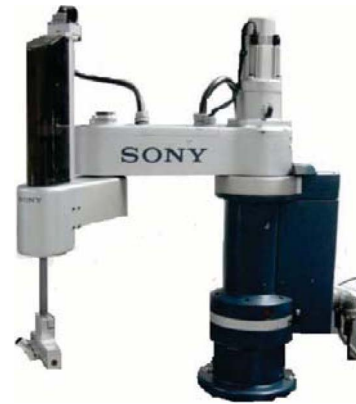
Fig. 8. SCARA robot controlled by the analog implementation of the control structure.
