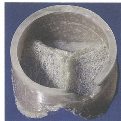
Fig. 4. Stented heart valve based on a non-woven PGA coated with 1% poly-4-hydroxybutyrate (P4HB) (17).
