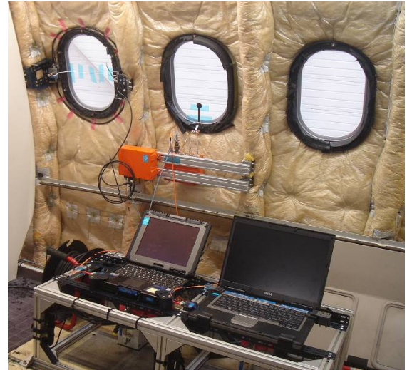
Figure 6. Installation of the test setup in the Airbus A340 aircraft. The leftmost window has the window sensor, the middle window the electric field sensor. The orange box is one of the sensor assemblies performing signal conversion and short term data storage. The laptops record all data during flight.
