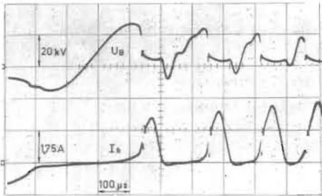
Fig.10.2.2. Load-break switch, I = 10 A (R.M.S.). Residual-current reignitions and new current-zeros due to main-circuit-oscillation.
