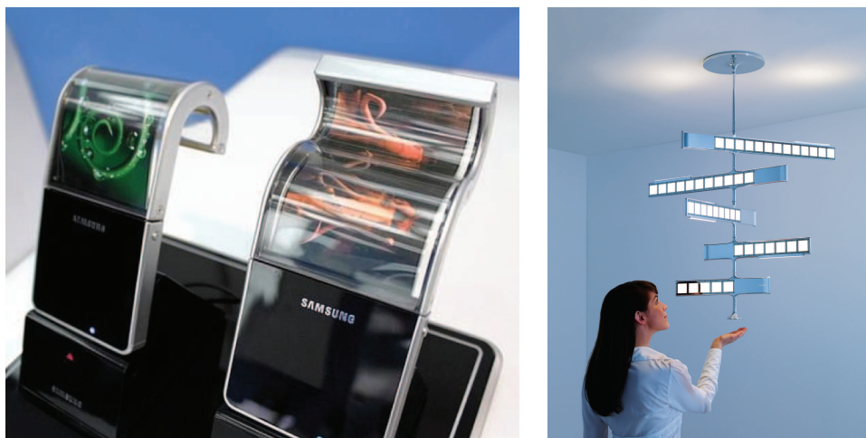
Figure 1.1 Two applications of organic semiconductors: (left) A flexible, very thin OLED display demonstrated by Samsung (© Samsung) and (right) decorative lighting from Philips 91 .
