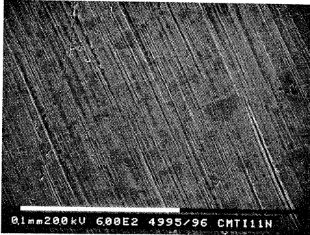
Figure 5.12 Undamaged tool surface of the reference lubricant (Cl-doped).
