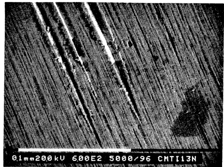
Figure 5.2 Abrasive wear; ploughing through softer contact partner
