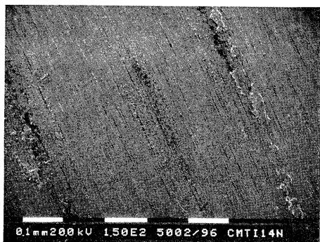
Figure 5.16 Survey of galled tracks, representative for most alternative lubricants
