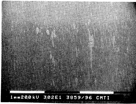
Figure 5.35 Failure of the TiAlN (z) coating and resulting adhesive wear
