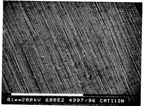
Figure 5.13 Tool surface comparable to the reference (lubricant 2)
