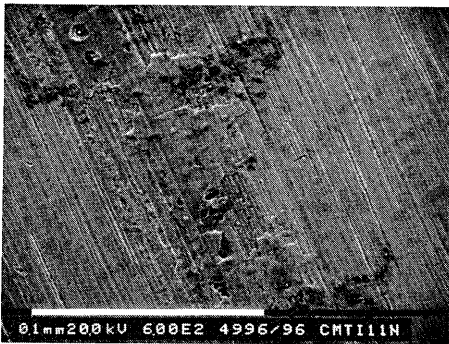
Figure 5.14 Incidental wear spot on the tool surface lubricated with the reference lubricant (Cl-doped)
