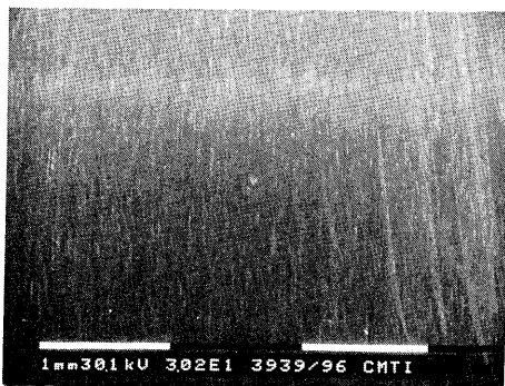
Figure 5.32 Hardly worn TiN (x)-coated tool after lubricated sliding to INVAR strip material
