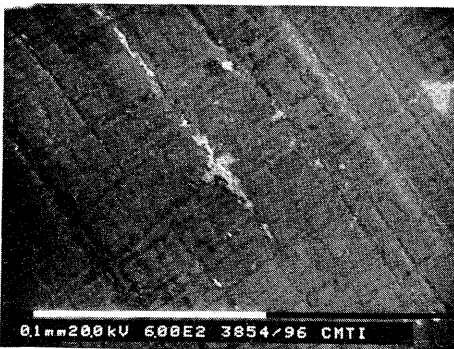
Figure 5.37 DLC-coated nipple with worn off upper coating (DLC) and micro scale adhesive wear on under coating
