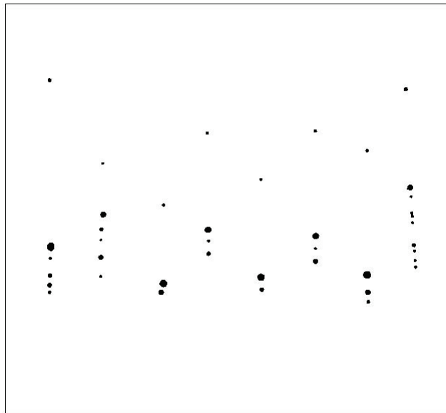
Figure 4.15: Printed bitmap using the standard pulse. The variation in the drop velocity results in a poor printing quality. The first drop is faster than the subsequent drops, several drops are merged together and form drops with large volume.
