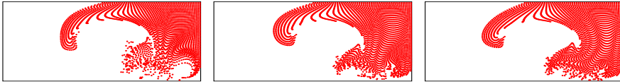
Figure 3.7: Simulated particle distributions for Re = 1 , 50 cycles (left), Re = 5 , 12 cycles (middle) and Re = 10 , 8 cycles (right).
