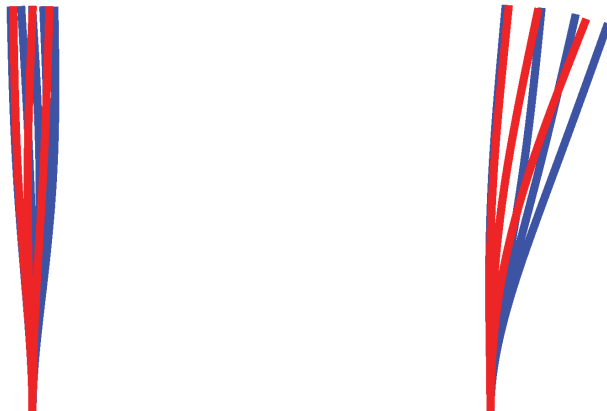
Figure 7.4: The forward (blue) and backward (red) stroke of a cilium in a Newtonian fluid (left) and the shear-thinning fluid (right). Both have the same actuation cycle with f_1 = 4 \cdot 10^5 \text{ Nm}^{-3} .
