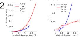
3. As hypothesized, a uniaxial fiber distribution was found for sample A and a uniform fiber distribution for B (left). Furthermore, the fiber tensile behavior of A was much more nonlinear (right).
