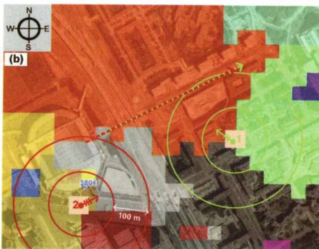
Figure 2. The layout of measurement site with (a) the grid of environmental classifications with open area (white), water (blue), vegetation (green), and urban (brown); and (b) the best-served areas for Base Station 1 (orange) and Base Station 2 (light grey), determined using the stochastic empirical propagation model discussed in Section 3.
