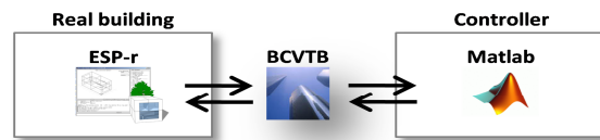
Figure 1: Design support environment for buildings with advanced building controls; BCVTB provides data exchange of sensor and actuator values between the building (ESP-r) and the controller (Matlab) during simulation run-time.
