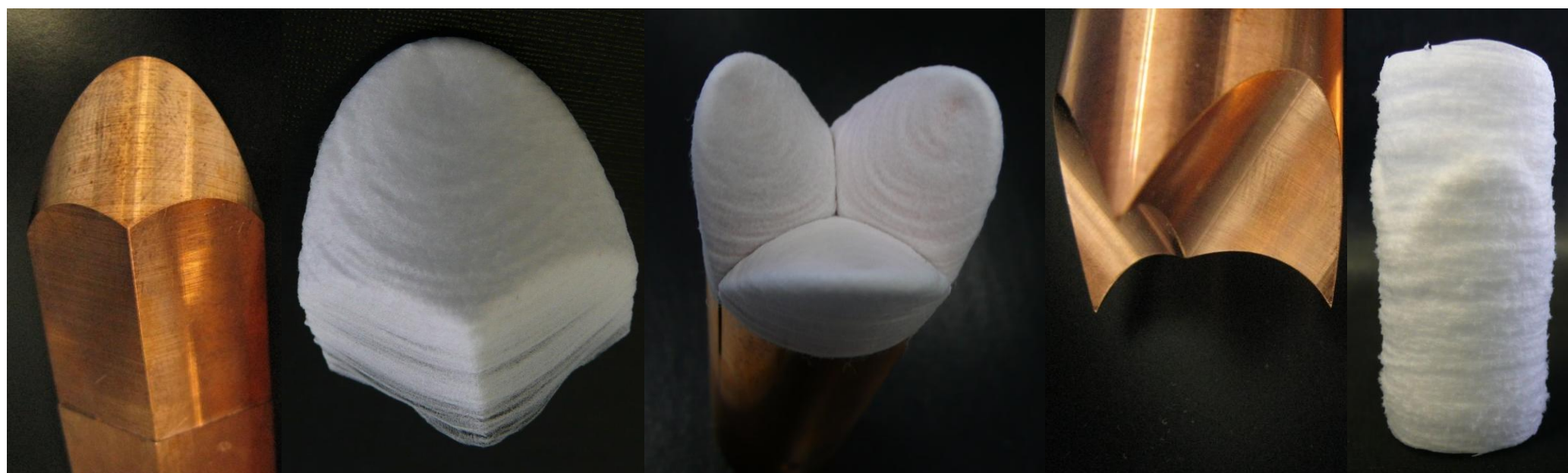
Figure 1 Process to electrospin a 3D valve starting with single leaflets
