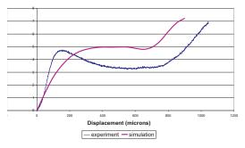
The finite element simulation for creasing process is in good qualitative agreement with experimental observations. However, quantitatively, the simulation deviates from experiments, specially in the post-buckling regime.
