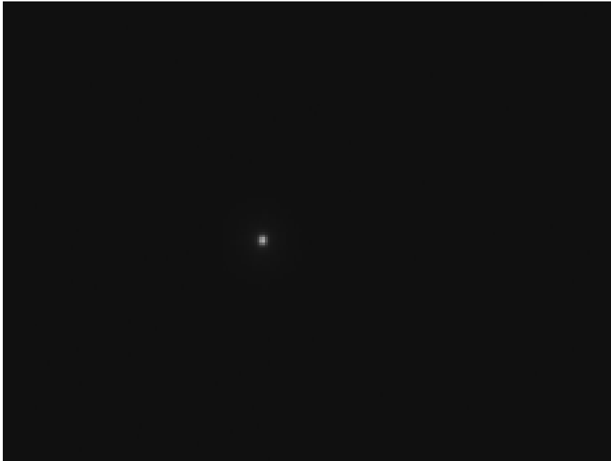
Figure 4.4: Electron spot on detector with no power fed to the cavity.
