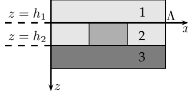
Figure 3.1: Geometry of the periodic model problem and division into layers.
