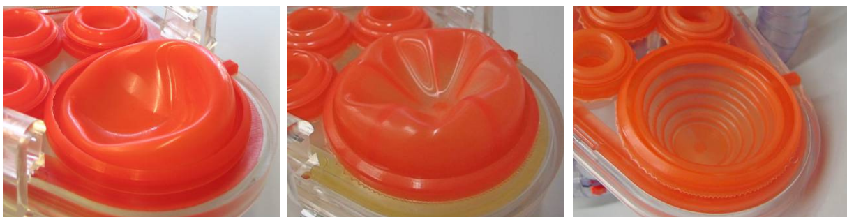
Fig. 2.6: Buckling of the three different bellow designs The first spherical membrane (left), the spherical membrane enhanced with five ribs (center) and the final membrane with a curled, wavy geometry (right).
