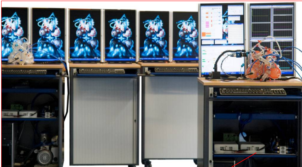
Fig A.2: The entire bioreactor set-up was reproduced four times. Every setup is build inside a mobile PC-working station
