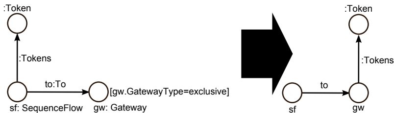
Figure 2: Graphical representation of a graph rewrite rule (attributed graph syntax)
