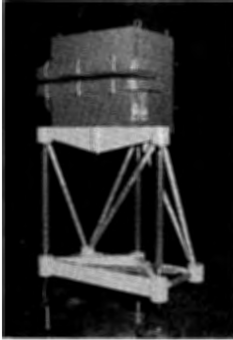
Figure 1: Dipole magnet and support system of the EUTERPE ring.
