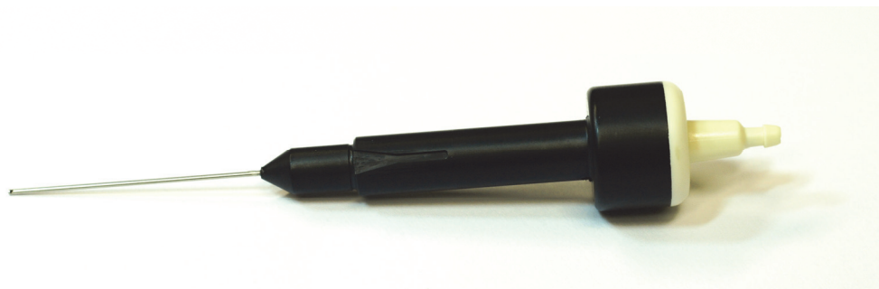
Figure 4.9/ Realized modified instrument: a vitrectome.
