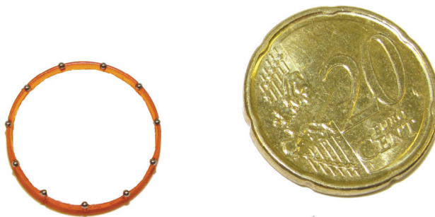
Figure 4.7/ Caged balls in a micro stereo lithographed cage, for the benefit of the \Theta -bearing.
