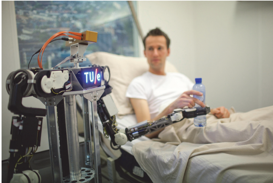
Figure 1.1/ The amigo care robot supplying a bottle of water to a patient [86].
