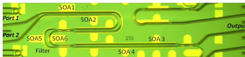
Fig. 2. Microscope image of the fabricated reconfigurable wavelength selector.
