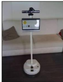
Fig. 1. The first version of the Florence robot.
