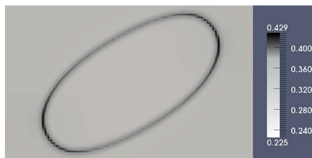
Fig. 8 Distribution of surfactant in a system of size n_x = n_y = 64 , n_z = 128 . The local surfactant density \rho^s(\mathbf{x}) is plotted on a 2D cut showing the centred x - z plane through a droplet sheared with constant velocity u_s = 0.06 and \rho_{\text{init}}^s = 0.25 ( Ca^{\text{eff}} = 0.16 ). The snapshot is zoomed into the droplet and as such does not accurately reflect confinement of the droplet or the elongation of the system. The surfactant accumulates at the droplet interface until saturation occurs. Compared to the remainder of the interface, a slightly higher local density is observed at the tips of the droplet (10 to 20 percent). This is caused by convection of the surfactant. 55
