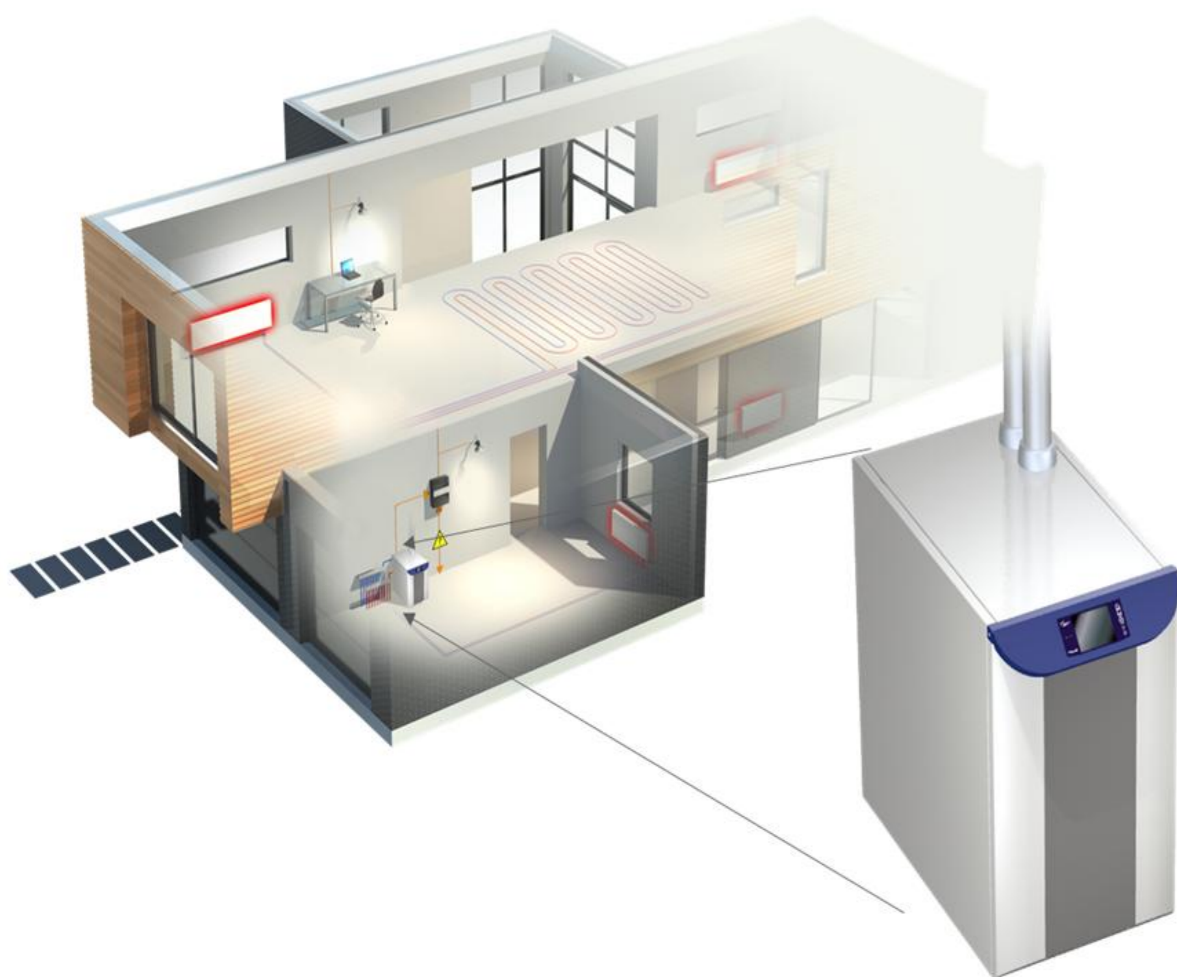
Figure 2 – Micro CHP system in a building
