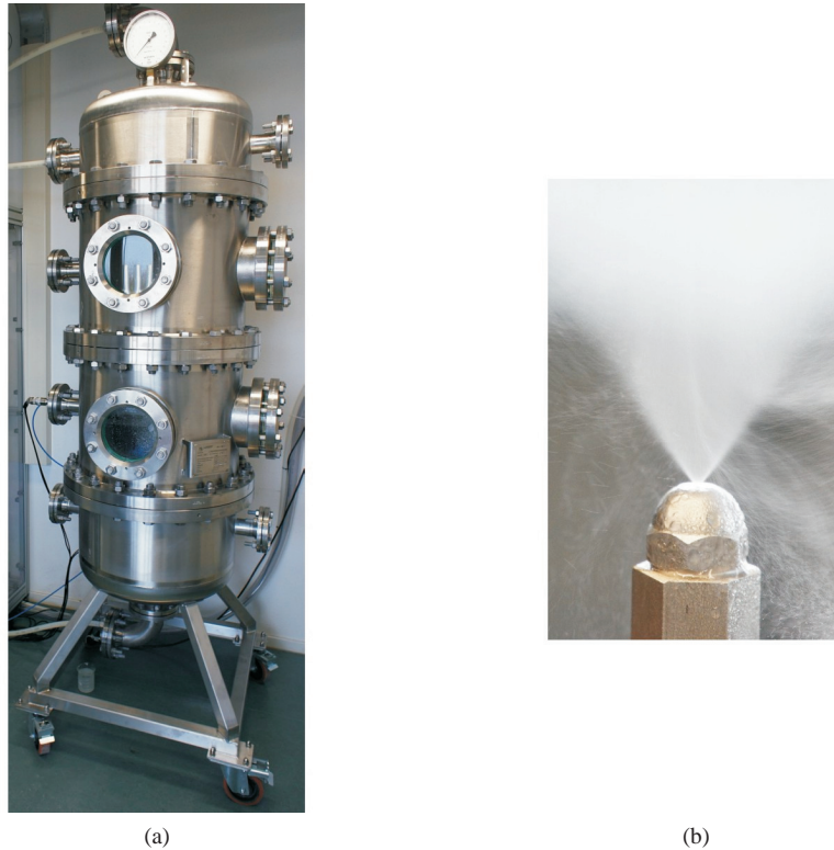
Figure 3.30: (a) The pressure vessel; (b) close up of a high pressure water nozzle that was used.
