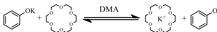
Scheme 2.2. The formation of a naked-ion phenolate nucleophile using potassium phenolate and 18-crown-6 ether as cation scavenger in DMA.
