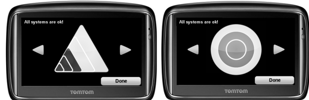
Fig. 3: HMI for deceleration (left) and acceleration (right)
