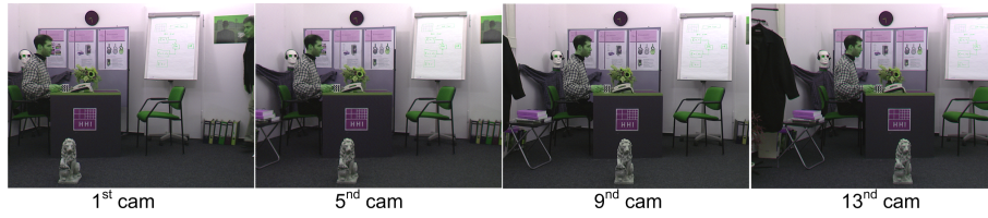
Figure 2.5: Thirteen multiple-view video streams captured by thirteen synchronized cameras as the input to the discussed depth estimation system.
