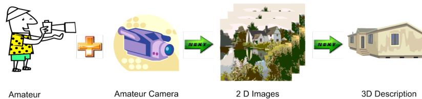
Figure 1.6: 3D modeling from video: a video of a large-scale scene is taken by a hand-held camcorder. The video is input to the scene reconstruction system and the 3D shape of the scene is reconstructed.
