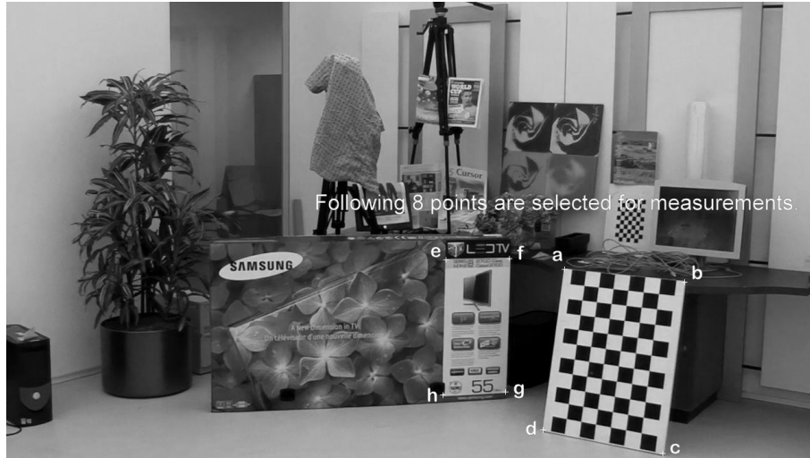
Figure 3.12: Eight points (a, b, \dots, h) are selected for measurement. The lengths of the eight line segments (l_{ab}, l_{bc}, \dots, l_{he}) and the eight corresponding orthogonal angles (\theta_{ad-ab}, \theta_{ba-bc}, \dots, \theta_{hg-he}) are measured for evaluating the accuracy of the reconstructed point cloud.
