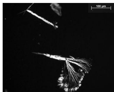
Figure S7. The optical micrographs of the sample of solution 8, obtained from 220°C superheated water for 60min. The concentration of Solution 8 was 30mg/ml. Crystals prepared from solution 8, appear to be dendritic in nature.
