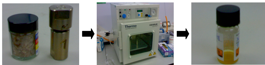
Figure S1. Sequence of pictures in which are shown the three steps of the “superheated water” treatment.
