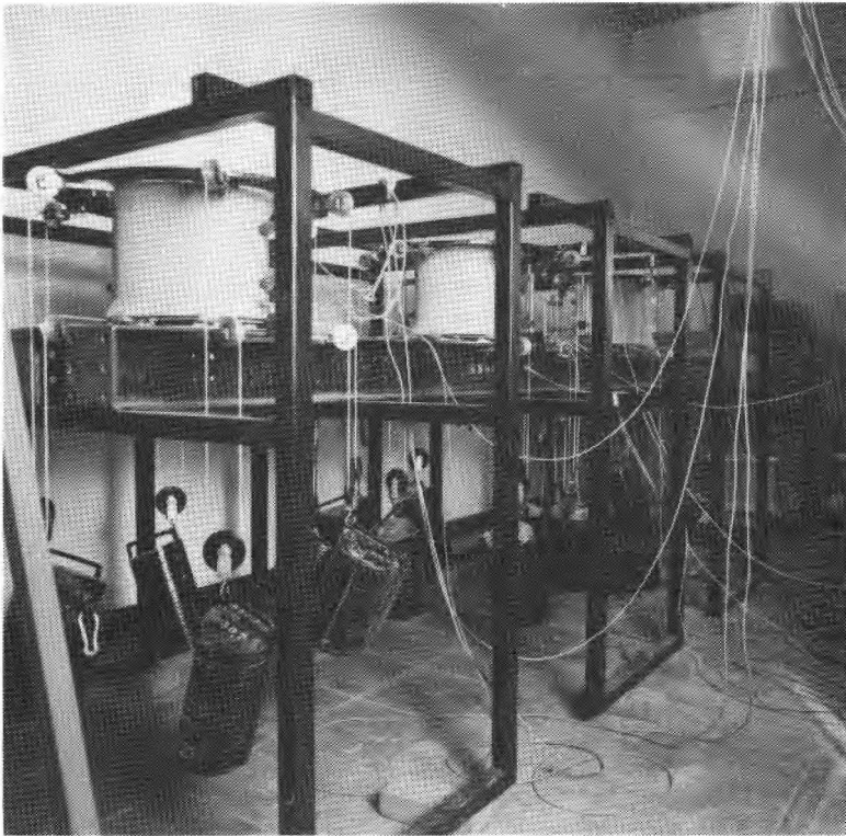
Fig. 6.13 General assembly of the long-term torsion creep testing rig.
