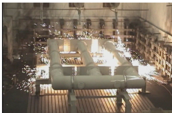
Fig. 16: Arcing by induced currents around generator bus duct in current withstand test at 850 kA peak
