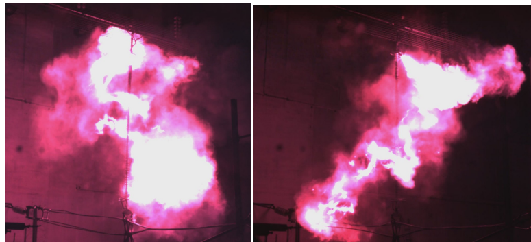
Fig. 12: 50 kA Power arc across string insulator, initiated by a small fuse wire. Left: Arc is burning between arcing horns. Right: Lower arc foot point formed on the OH line
