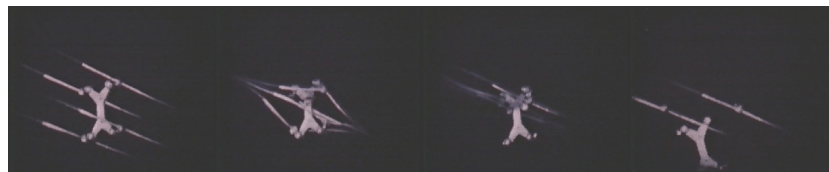
Fig. 13: Bundle contraction and expulsion of line spacer due to high short-circuit current in a test (50 kA, 0.3s)
