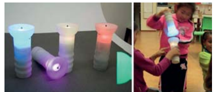
Fig. 28: ColorFlares. Tilde Bekker et al. (TU/e). These play objects change color when touched or rolled and start to flash if you shake them. The toys enable the children to come up with their own rules or game scenarios, which depend completely on the context such as indoor, outdoor or as part of another game.
