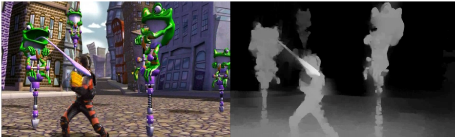
Figure 25. Screenshot of the content. The content is stored in the WOWxv 2-D-plus-Depth format, i.e., a red-green-blue (RGB) image (left) with a corresponding depth map (right).
