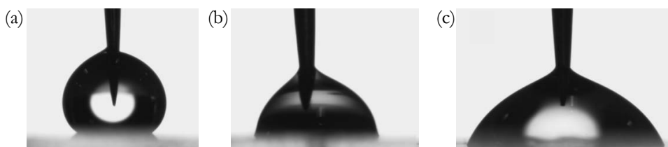
Figure 5.6: Side view of water drops during electrowetting experiment on a corrugated surface. The needle is seen inserted from the top. (a) The Cassie-Baxter (suspended) drop at 0V before actuation, with a base radius of approximately 1\text{ mm} . The Wenzel (collapsed) drop at 150V during electrowetting, viewed (b) perpendicular and (c) parallel to the grooves. The elongation of the drop parallel to the channels is clearly visible from the difference in base length and contact angle between (b) and (c).
