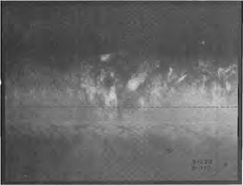
Figure III.15. Detail of figure III.14. P-Si region showing some resemblance to the lens shaped p-Si structures found in the Cu implanted material after annealing at 0.44 \text{ Jcm}^{-2} (figure III.9). The dashed line indicates the calculated melt depth of \approx 180 \text{ nm} .
