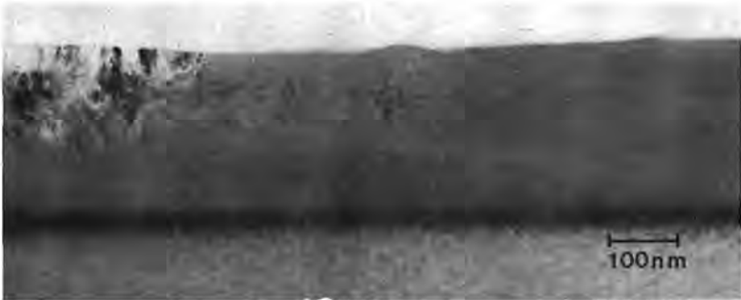
Figure III.8. Detail of a p-Si patch at 0.44 \text{ Jcm}^{-2} . The structure exhibits a large wing centered around the buried Cu layer.
