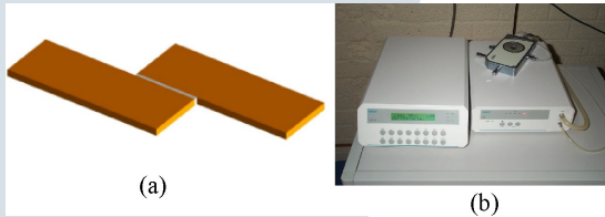
Figure 1 (a) Configuration of solder specimen and (b) Linkam heating-cooling stage.
