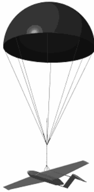
Figure 20.5: The SensAir UAV with deployed emergency parachute
