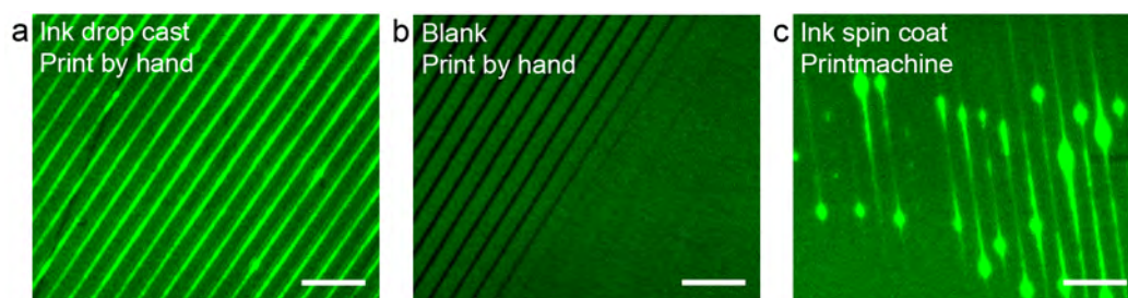
Figure 6.9: CLSM images of PEN films patterned in three different ways, all recorded with the same settings. Trenches in b are black due to the small focus depth of CLSM. Scale bars represent 10 \mu\text{m} .
