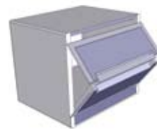
Fig. 10b Wall Oven: a split folding door enables hot surfaces to mate and minimize reach-over length. This can reduce accidental burns and would provide a surface at counter line to slide out hot cookware.
