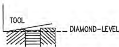
Fig.4.6. The surface roughness caused by the anisotropy of material behaviour.
