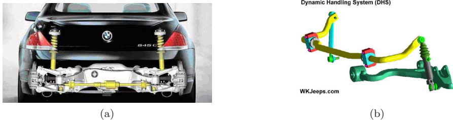
Figure 1.1: Commercial active anti-roll bar control systems. A rotary equivalent with the actuator situated in the middle [6] is shown in (a), where (b) shows the linear variant [7] with the actuator situated on the right in the picture.
